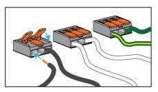
Terminate EchoConnect wiring using provided WAGO connectors.
